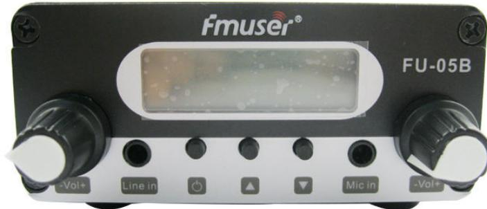
CAUTION: NEVER operate the transmitter without connecting a suitable antenna or dummy load to the output otherwise there is a serious danger of destruction of the output stage of the transmitter.
