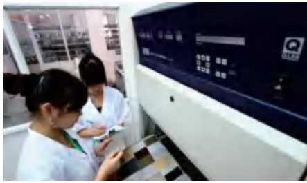
氙灯人工气候老化仪 Q-SUN Xenon Test Chamber
